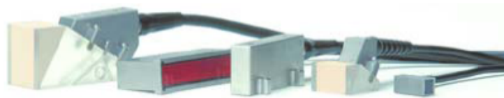
Figure 1-3 Typical phased array probe assemblies
